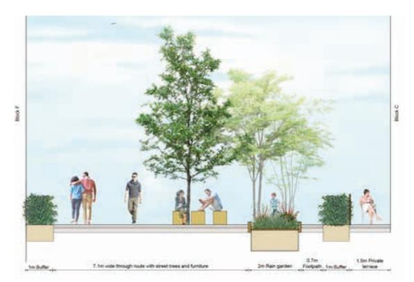
Section AA. Sketch section showing the relationship between a residential terrace and the public realm with buffer planting and rain garden providing a lush environment and separation
